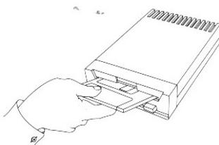
Disks should be inserted into the drive metal-end first with the labeled side facing up. To remove a disk, simply press the button on the lower, right side of the drive. Always wait for the disk drive light to go out before removing a disk.
