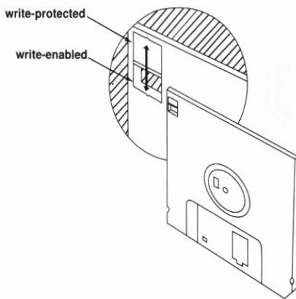
When the tab is in the upper position and you can see through the hole in the disk, you cannot change any information on the disk. To be able to save or delete information on the disk, make sure that the tab is in the lower position, covering the hole. This is known as the *write-enabled* position.
